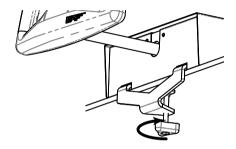
**2.2.** If you want to set up the YOKO/YOKO+ in your custom home cockpit, you can use the included clamping knobs (D) to screw it to your support base. For more detailed measurements and customized setups, visit our help center (help.virtual-fly.com).
