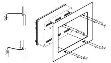
To mount the PFD/MFD to your custom flight panel from the back, your panel will need a cutout that matches the measurements depicted in the blueprint below. All measurements displayed are in millimeters.
